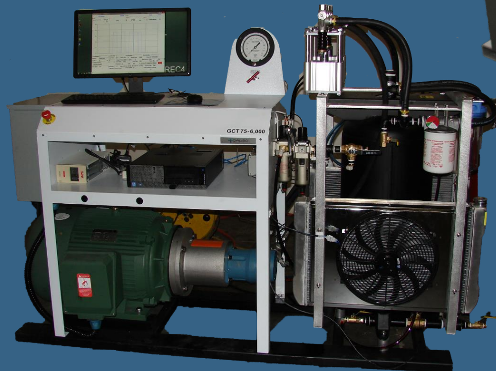
GCT75-6k Pressure:6,000psi Flow: 17.2gpm Medium: Oil
